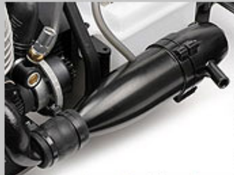
Dual-chamber aluminium tuned pipe gets more power from the engine
