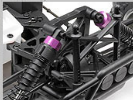
Long-stroke oil-filled shock absorbers tame the roughest terrain
