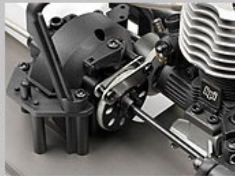
Fibreglass disk brake provides strong deceleration and good durability
