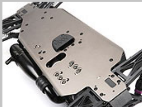
2.5mm thick cool anodised aluminium chassis
