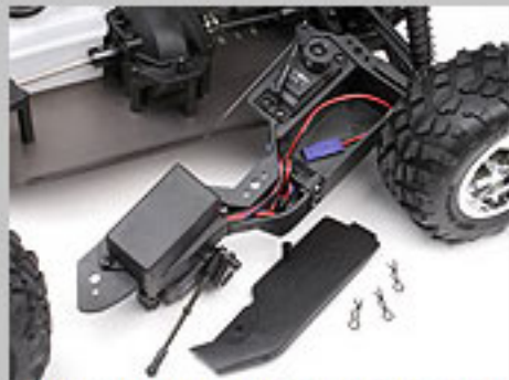
Removable radio tray for easy maintenance and cleaning
