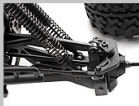
Heavy duty double wishbone wide track suspension handles even the roughest terrain
