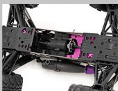
Shaft driven 4 Wheel Drive for best traction on all surfaces
