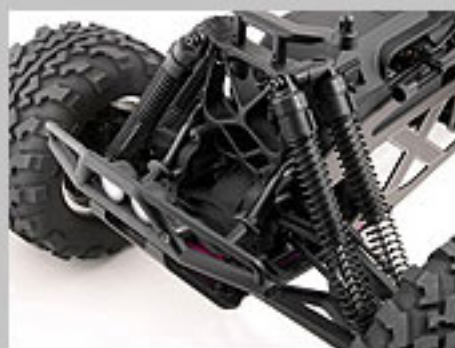
8 long stroke oil filled shocks with firm tuned springs keep the wheels on the ground
