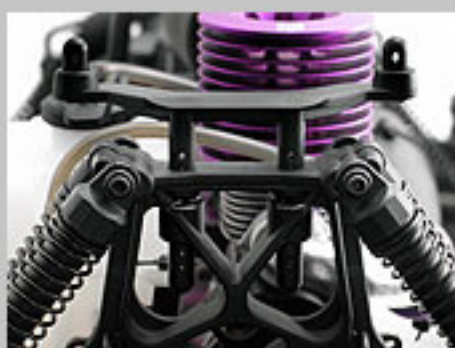
Adjustable body post for easy mounting of optional bodyshells
