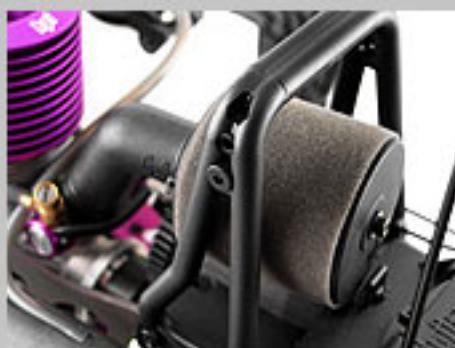
anti roll bar to protect the chassis and engine
