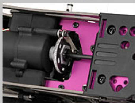
Adjustable fibre disk brake for efficient deceleration and precise "in air" control
