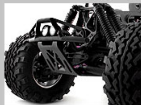
Front & rear skid plates for impact protection
