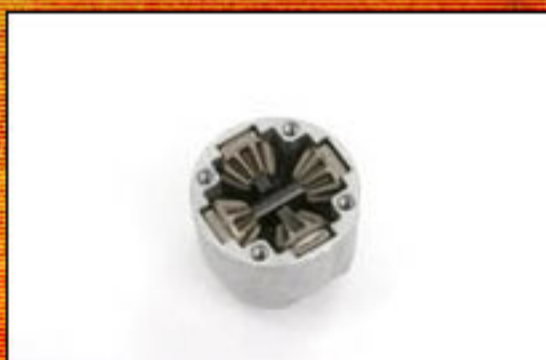
Shimmed spider gears, pinion gears, diff case bearings
