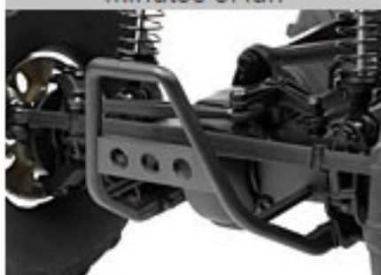
Strong front bumper to protect drivetrain
