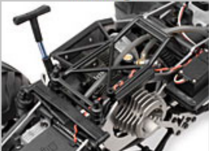
Unique chassis design with laydown engine
