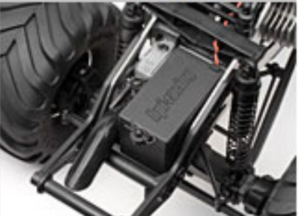
Rear-mounted battery box for wheelie stance
