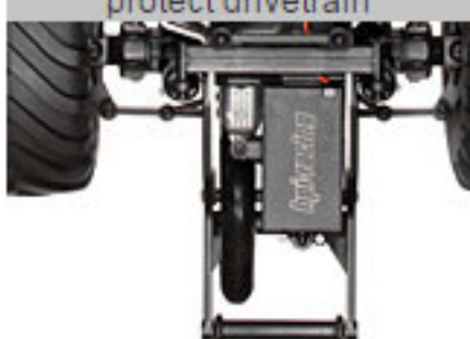
Wheelie bar for controllable cool wheelies
