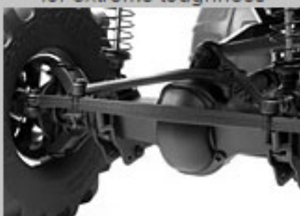
Extra-tough solid axles for simplicity and ruggedness
