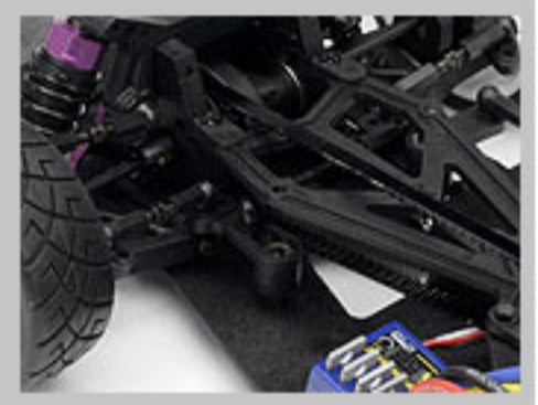
New redesigned chassis, new chassis plate & new top deck
