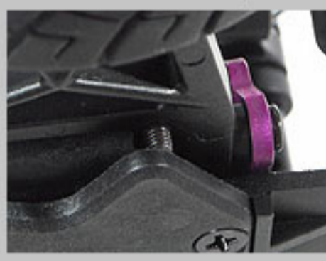
Adjustable droop - Better handling and tunability especially on high grip tracks
