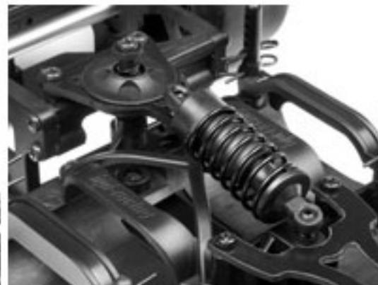
Friction damper FRP T-bar features high traction. Roll amount can be adjusted by tightening the screw.
