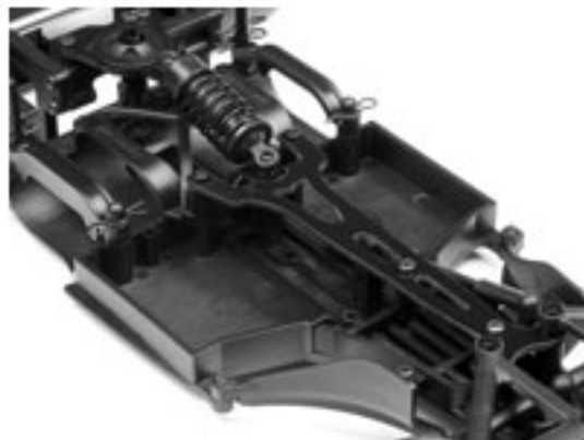
FRP upper deck to reduce pitching and stabilize drive performance
